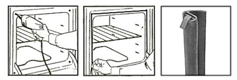
Measure hole to hole dimensions and choose appropriate gasket length from the available selection. The replacement gasket stretches between and mounts into the holes created, using the gasket retaining clips factory installed onto each end of the gasket.
